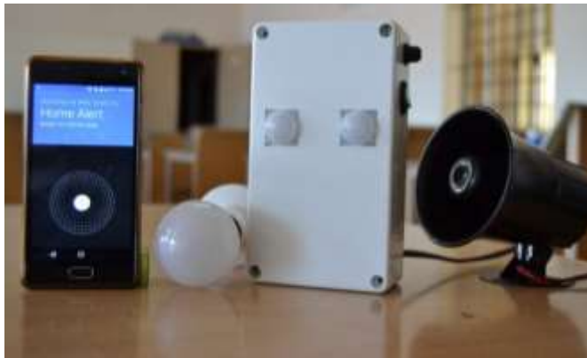
Model 1: capable of making a phone call to alert the owner
