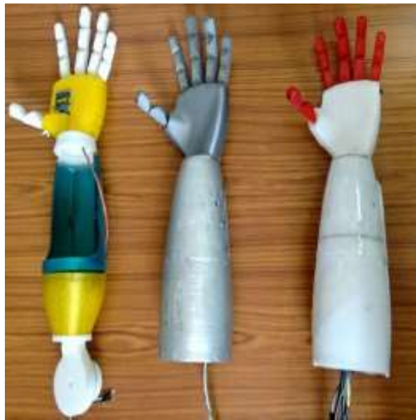
Indigenously built prosthetic Arm using 3D printer
