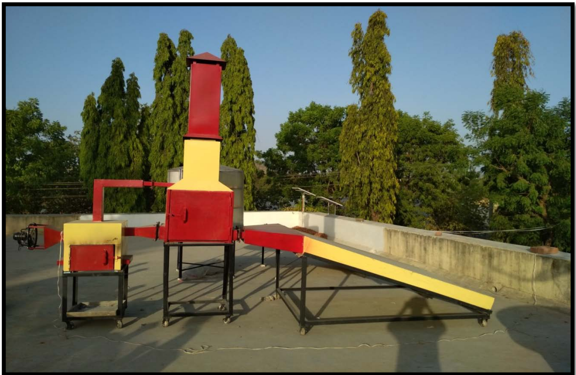
Fabricated solar cum biomass powered hybrid dryer
