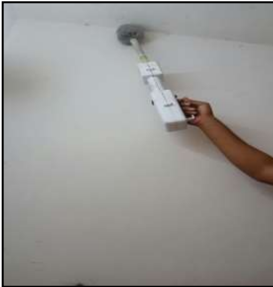
Photograph 1 The developed Prototype model cleaning the cobweb on wall
