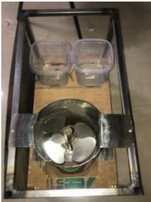
Internal Design of Bio-Waste Cutting, Dehumidifying and Compost making Blocks
