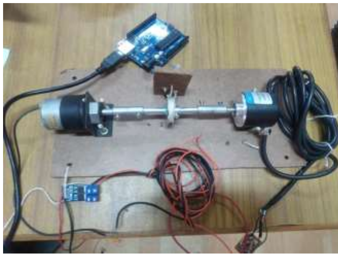
Fig. 5: A rotary encoder coupled with a DC Motor
